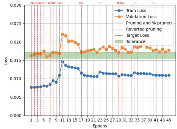
Fig. 4. Training and validation loss during the adaptive pruning process using the **global** approach.
